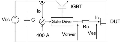
Fig. 1 Schematic of short-circuit test circuit for MOSFET
