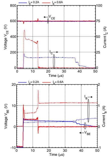
Fig. 3 Failure of BJT for  $T_{CASE} = 25^\circ\text{C}$ .
