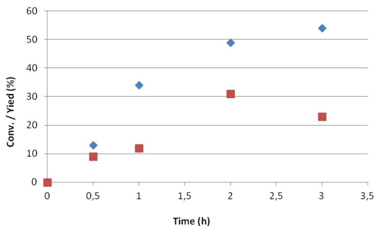
**Figure 1.** Conversion of aldehyde **2** (% , blue diamonds) and yield of aldolization product **3** (% , red squares) over time. Conditions: 60°C under microwave irradiation.
